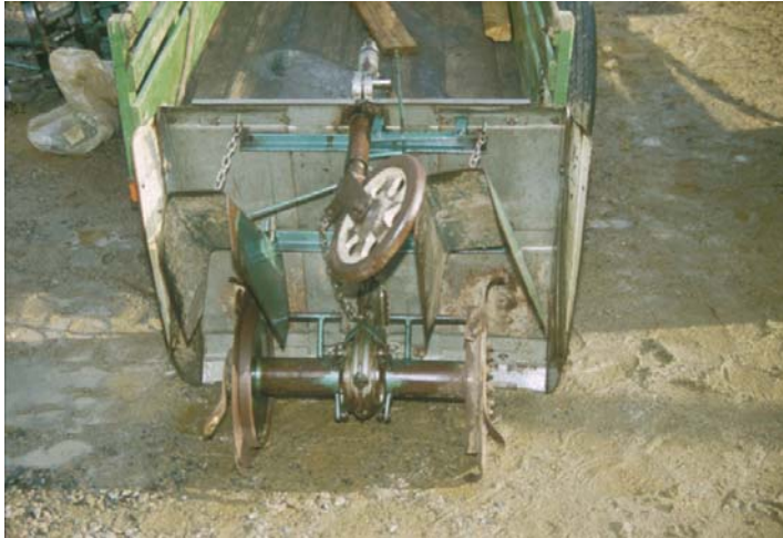
Plate 24 Working elements of a power tiller furrow opener. (T. Friedrich)
