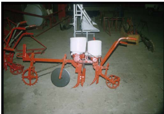
Plate 25 Planter with hoe openers for fertilizer and seed following the cutting disc. (T. Friedrich)
