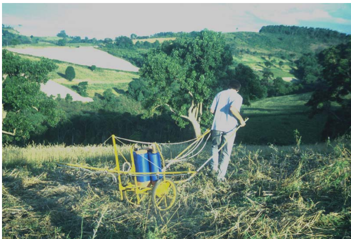
Plate 14 An adapted knapsack sprayer for manual traction. (T. Friedrich)
